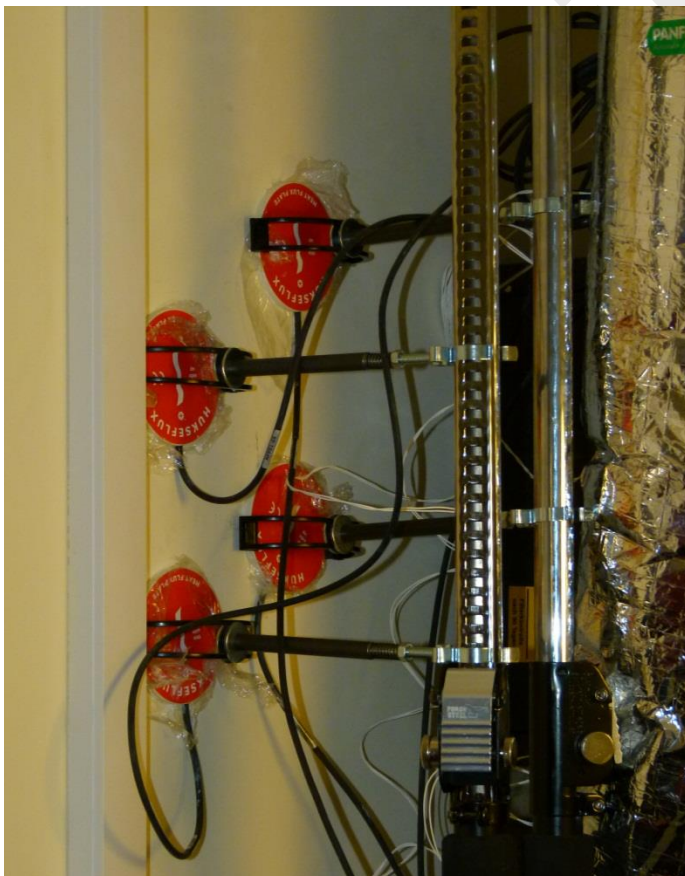
Figure 8: Heat flux sensors 'placed' against the wall
